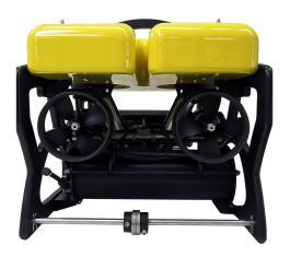
The **Steelhead** inspection-class ROV is a portable, lightweight and stable underwater system that is easily operated through intuitive flight controls. Its small profile allows this vehicle to inspect confined spaces and be easily stowed.
